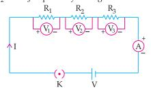
Total Potential,  $V = V_1 + V_2 + V_3$
