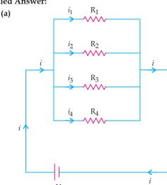
Let there be n resistance, each of value  $R_1, R_2 \dots R_n$  respectively connected in parallel to a battery of voltage V.
