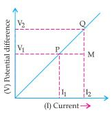
The slope gives the resistance of the resistor used in the circuit.
