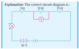
2. How much is the total resistance in the above circuit diagram?
